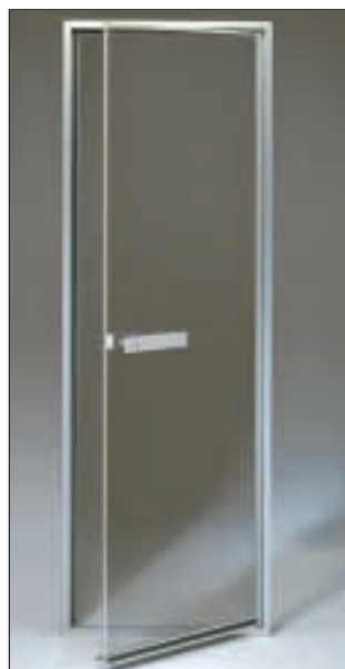
Steam Door 50 G (Art. no. 9091 1010) Elegant model in tempered clear glass with concealed hinges. Magnetic strips for a tight seal. Stainless steel edging round door leaf, drainage strip and air-vent. Frame size: 185.5 x 63.5 x 4.3 cm. Opening width 55 cm.
