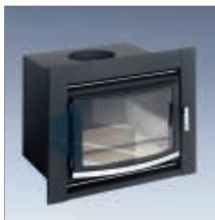
TS-12 (Art. no. 6505 1000) With bowed glass door. Designed for smaller fireplaces. Front measures 405 x 400 mm. Straight body, depth 400 mm. Door may be hung to open left or right.
