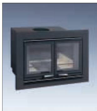
TS-26 V (Art. no. 6505 1040) With two glass doors – a practical solution when space in front of the fire is limited. Comes complete with practical ash-pan and adjustable grate. Front measures 528 x 480 mm. Straight body, depth 470 mm.
