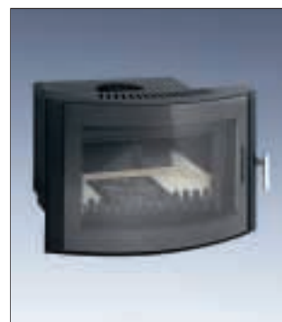
TS-77 V (Art. no. 6505 1090) Exclusively designed fire insert with a large, bowed glass door, ash-pan and adjustable grate. Front measures 530 x 480 mm. Straight body, depth 440 mm. Door may be hung to open left or right.
